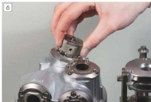
Putting on the secondary clearance.
